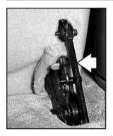
4. While holding the seat forward, pull the support rod out from the retainer clips and flip it down until it latches into place.
